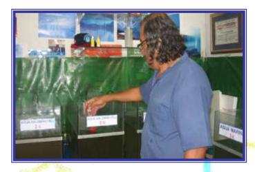
In order to eliminate the residues from the bottom, the bottom of the aquariums was siphoned every other day, renewing 10% - 20% of the water. The cleaning of the pumps was done in the same interval of time.
