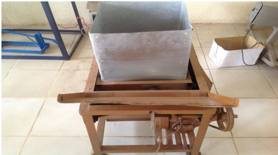
Fig. 4. Garri sieving machine showing the detachable hopper
