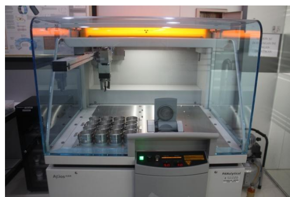
Figure 4. XRF equipment used for whole rock chemical analysis in this study.
