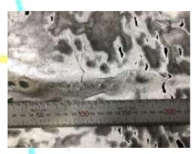
Fig. 7 Solidification cracks
