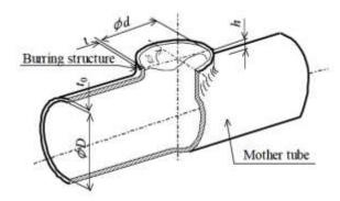
Fig. 1 Overview of branch pipe [2]
