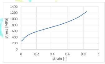
Fig. 3 Deformation resistance obtained from experiments
